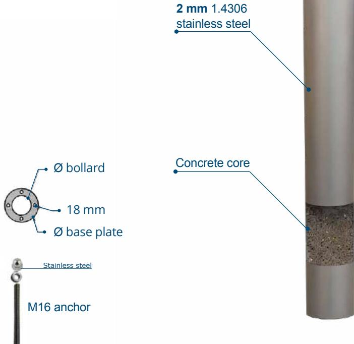
**1** Stainless steel bollard for core drilling
